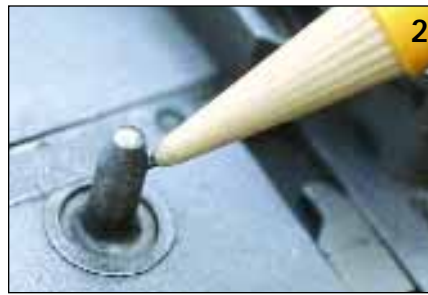
The E in this Model 629-2E (1) stood for "Endurance" package wherein guns were reengineered to last longer. Some of the Endurance package changes (transitioned between 1988 and 1990) included: (2) radius stud package, (3) bolt block, (4) lengthened cylinder stop notches and a special heat-treated yoke (not shown).
