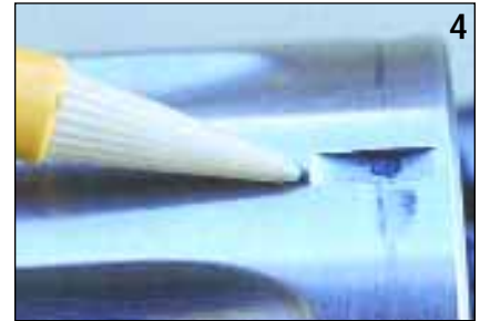
The E in this Model 629-2E (1) stood for "Endurance" package wherein guns were reengineered to last longer. Some of the Endurance package changes (transitioned between 1988 and 1990) included: (2) radius stud package, (3) bolt block, (4) lengthened cylinder stop notches and a special heat-treated yoke (not shown).
